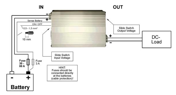
First connect the DC-DC converter, after that the battery.
