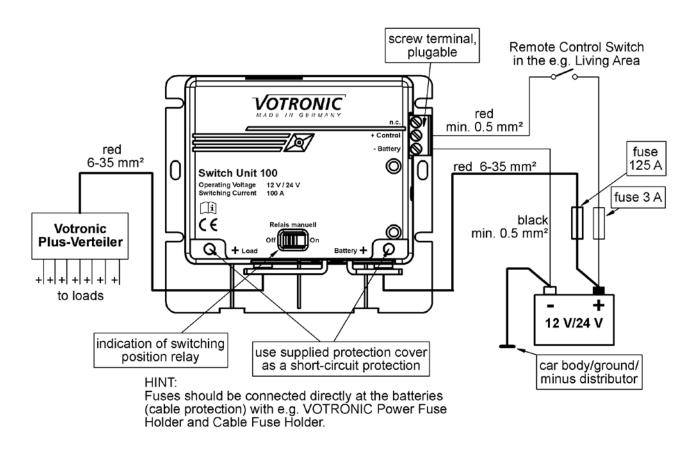
This application example enables through a switch in the living room the remote-control of the product. Current consumption of the unit is only 0.003 A, therefore a miniature switch is sufficient.
