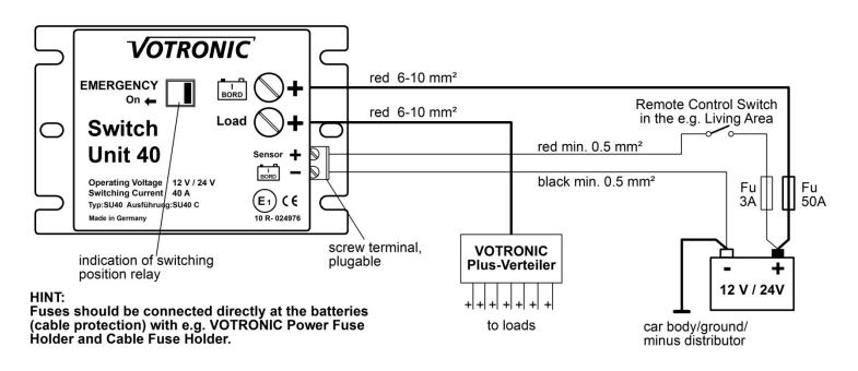
This application example enables through a switch in the living room the remote-control of the product. Current consumption of the unit is only 0.002 A, therefore a miniature switch is sufficient.
