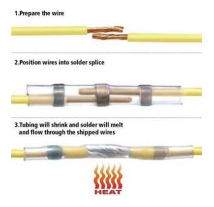
The advantages of this connector are that the shrink tube effect makes the connection insensitive to oxidation, water and dirt and the stabilizing effect of the shrink tube makes this solder connection absolutely uncritical in mobile use.
