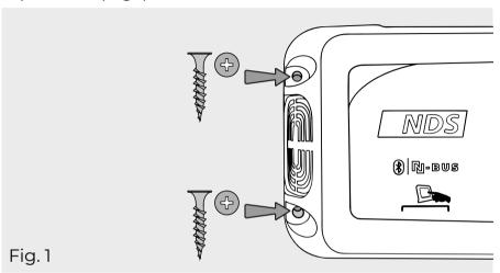
All electrical and setup connections are on the front, it is not necessary to disassemble the plastic shells, except for the protection fuse replacement.
